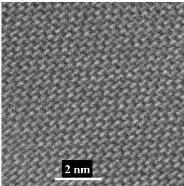
Fig.1 Transmission electron microscope image of  $\text{Cd}_{3-x}\text{Zn}_x\text{As}_2$  ( $x = 0.13$ ).
