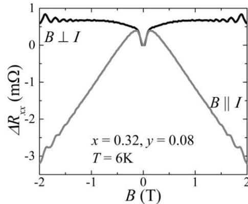
Fig. 2 Transverse and longitudinal MR of the  $(\text{Cd}_{0.6}\text{Zn}_{0.32}\text{Mn}_{0.08})_3\text{As}_2$  sample at 6K.
